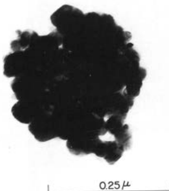
Fig. 12-54. A single Type 107 image aggregate at high magnification. Aggregates average 150 to 300 nm in diameter, and each comprises about 40 closely associated fine particles, which are individual crystals of silver.
